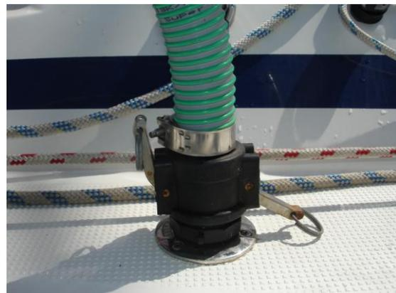
Figure 3: Pumpout hose connected to deck fitting via Camlock Coupling
