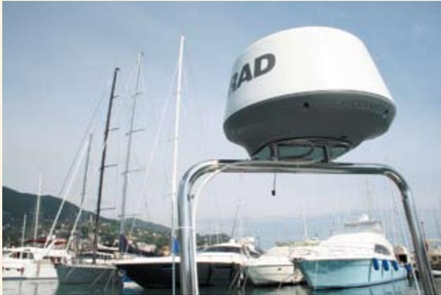
There are two microwave antennas (one on top of the other) inside the antenna dome of the Navico Broadband Radar. One transmits while the other receives, unlike a conventional radar that only has one antenna used alternately to transmit and then receive.
